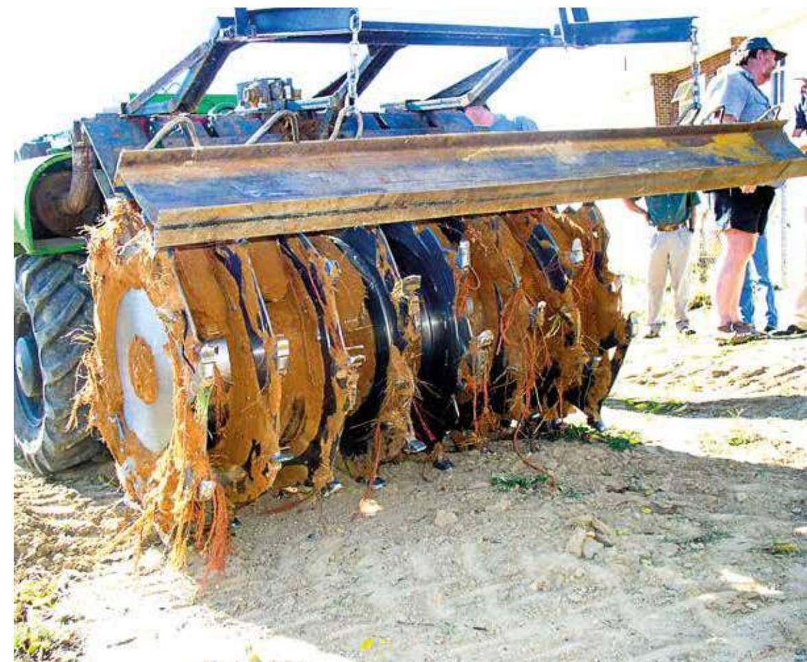
FIGURE 1. Soil mix implement used for soil preparation at Kanonkop.
