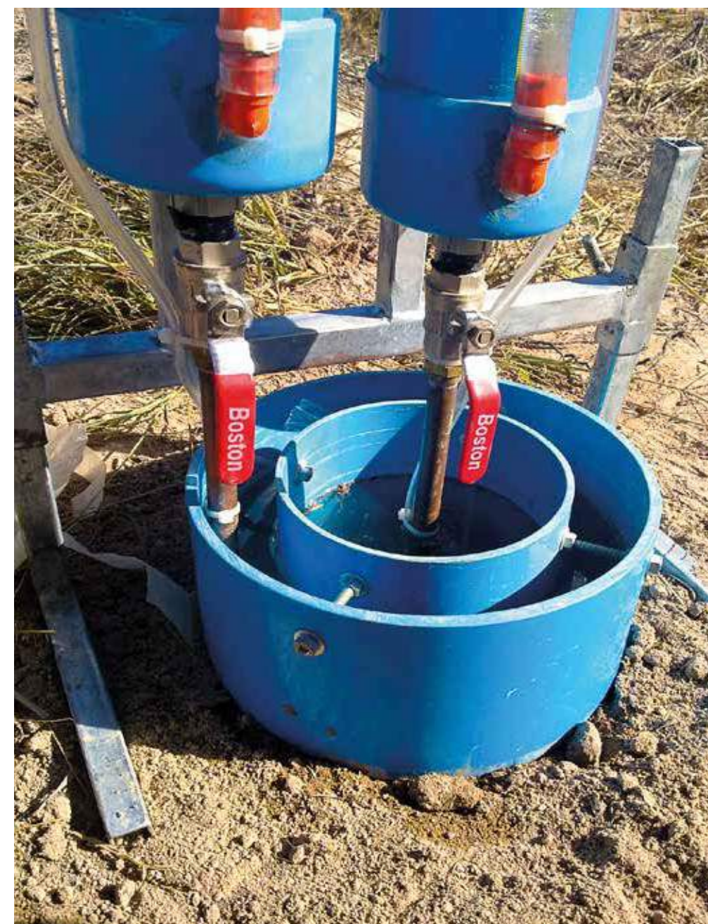
FIGURE 3. Double-ring infiltrometer for determination of saturated hydraulic conductivity.
