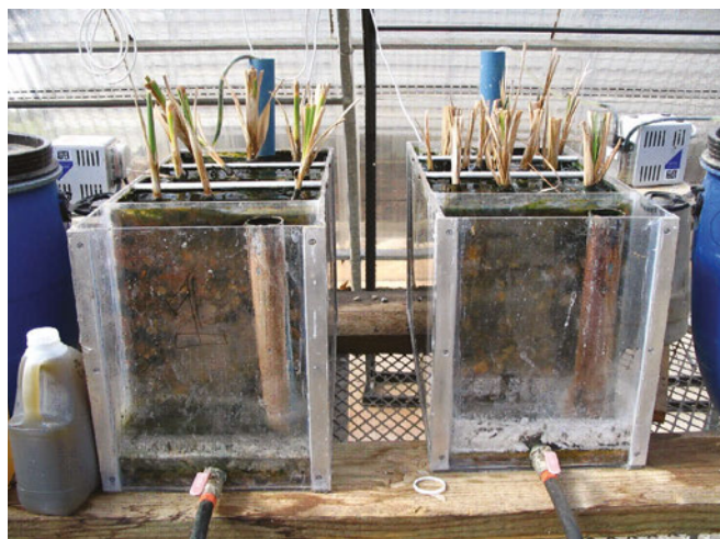
FIGURE 1. The experimental wetland systems at the start (left image) and end (right image) of Trial 3. In each image, the control wetland is on the left and the ozone pre-treated wetland on the right. Note the greater height of the Phragmites spp. in the ozone pre-treated wetland.
