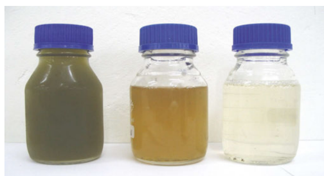
FIGURE 2. Effect of passage through the wetland, and of post-wetland ozonation on ozone pre-treated distillery wastewater. Left, wastewater prior to entry into the wetland. Centre, the same wastewater after it had passed through the wetland. Right, wastewater after it had passed through the wetland and undergone post-wetland ozonation.
