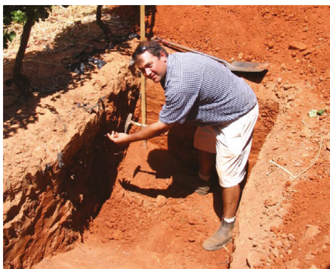
FIG 5: This profile pit at Darling has a neat walk-in space and is wide enough to turn around in so that one may study soil preparation and root growth, as demonstrated by Leon Dippenaar at the 2006 Swartland vineyard block competition. The profile, however, could have been deeper and closer to the vines (300mm).
